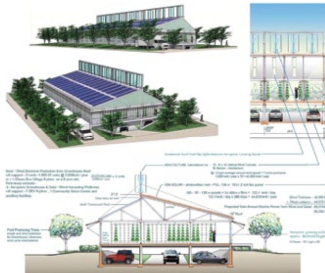
Hydroponic-Aeroponic Solar-Wind Greenhouse , 2007
